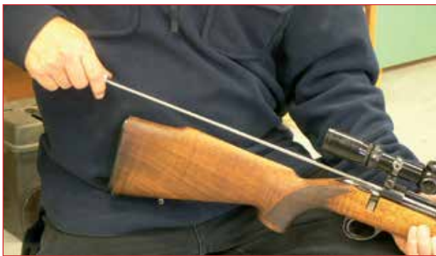
Figure 8: Cleaning a firearm. The rod is inserted from the chamber end of the barrel.
